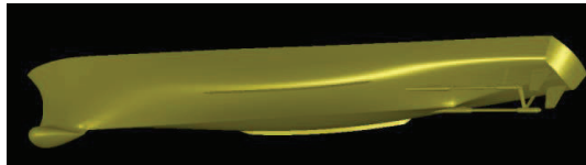
Fig. 1: Combatant ship David Taylor Model Basin (DTMB) model 5415
